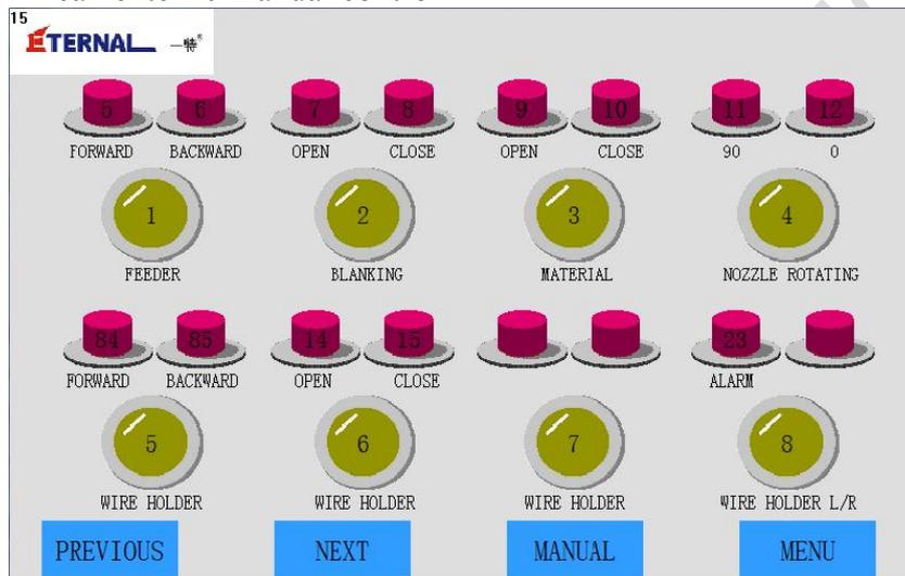
Click the yellow button to control the corresponding cylinder to open and close the action. The red indicator refers to the trip detection of the cylinder in the open and closed mode. The detection in this case must be written to the program when editing the program, and each output has one or two Input tests.
