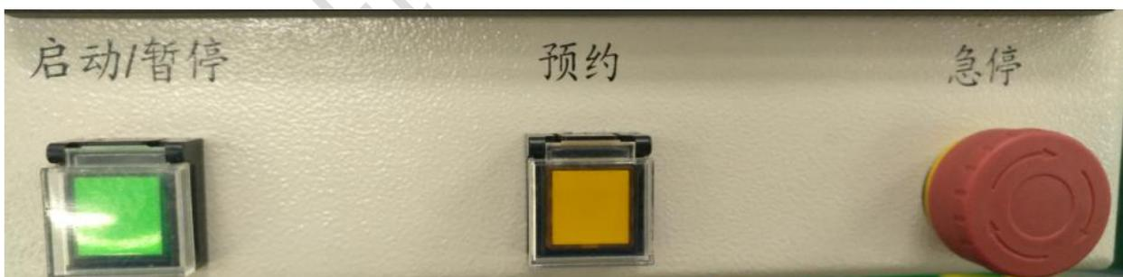
**Start:** this is the start button of the program, in the state of zero completion, press this button, the winding machine will start action.
